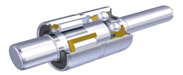
The special double row bearings built not separable and sealed unit. They are composed of a schaft and cylindrical bushing which is arranged in two rows of rolling elements. The rolling elements are seated in light single-sided plastic cages. The raceways on the shaft and in the cylindrical bushing are produced with a very high degree of accuracy. In order to protect them against penetration of impurities, they are equipped on both sides by efficiency contact sealing.
